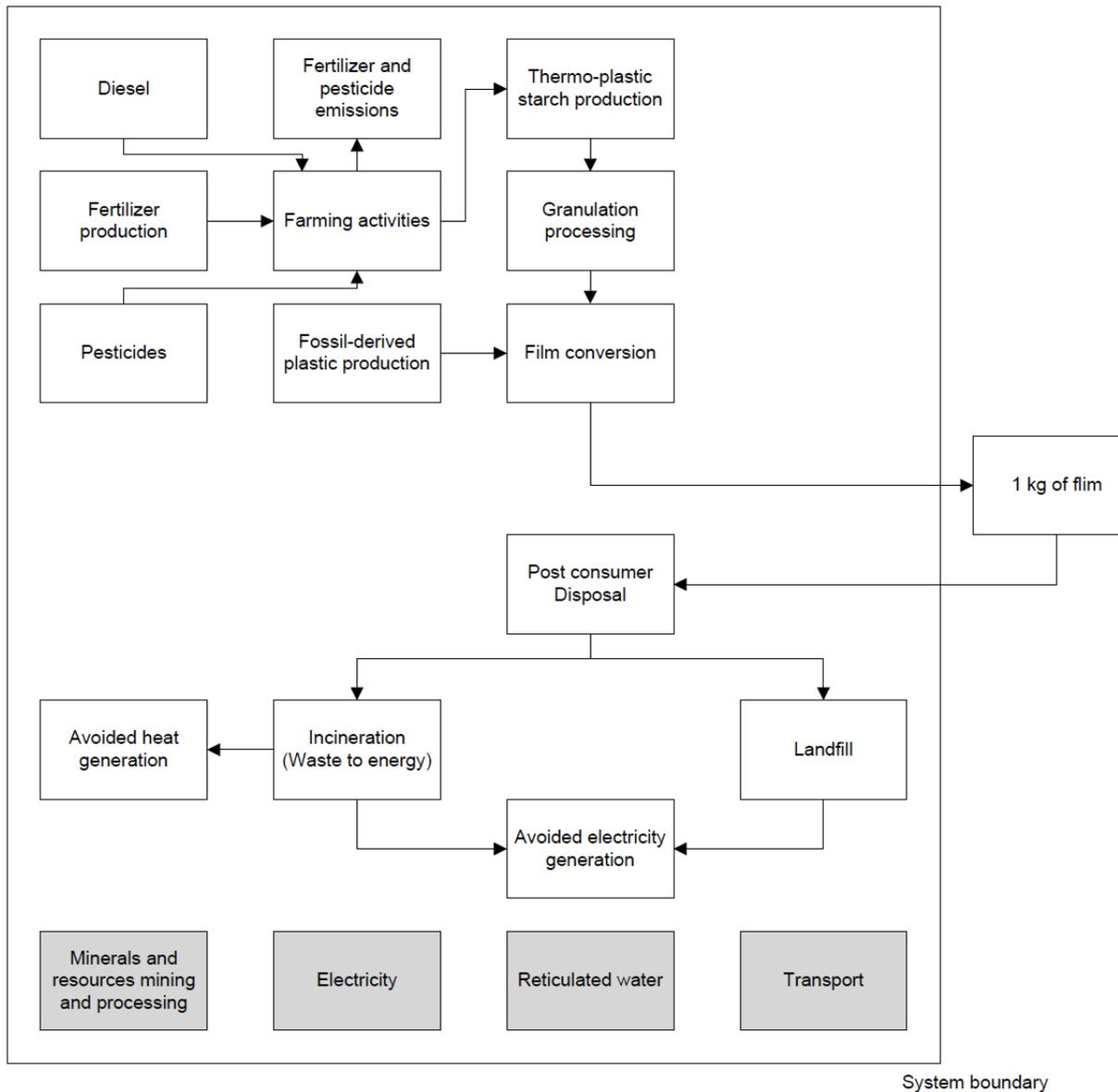
**Figure 1.** Diagram illustrating key processes considered in LCA
